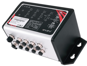
LNP-0800G-M12-67-24(-T) 8-Port Industrial M12 IP67 Waterproof Gigabit PoE+ Ethernet Switch, w/8*10/100/1000Tx (30W/Port) M12 Connectors (X-Coded)
