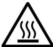
Figure 1.2 - Hot Surface Warning Label
