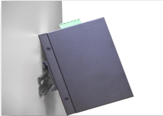
Figure 3.2 - Insert the Switch on the DIN-Rail
