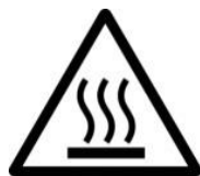
Figure 1.2 - Hot Surface Warning Label
