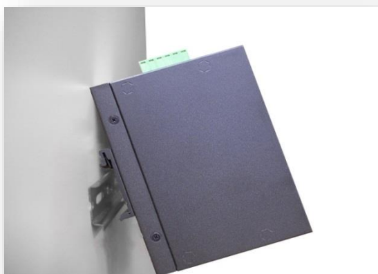
Figure 3.2 Insert on the DIN-Rail
