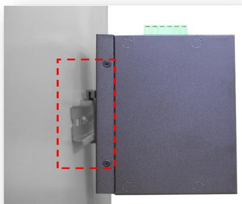
Figure 3.3 Secure on to the DIN-Rail
