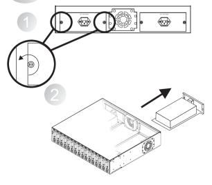
Turn off screws from the two sides of power supply then pull power supply out.
