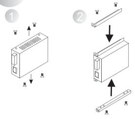
When installing media converter into the Chassis.
