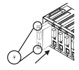
Push media converter into 16 Slots Universal Media Converter Rack and fasten screw on the slider of media converter
