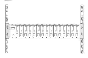
Fasten screws in rack to fix 16 Slots Universal Media Converter Rack
